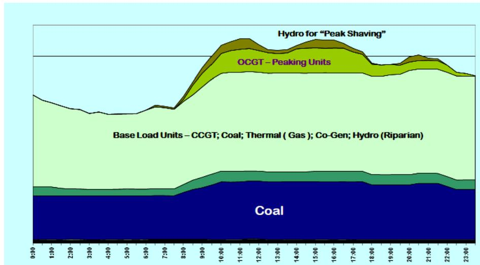
Figure 1: Energy Generation Dispatch by Fuel Type for Typical Daily Load Duration Curve Characteristic (Peninsular Malaysia)
